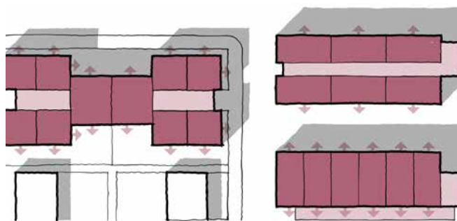
Figure 119 Diagram illustrating buildings orientation designed to maximise sunlight and shading. Source image: National Model Design Code
