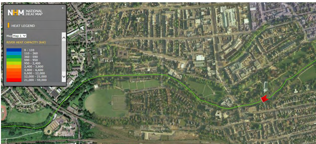
Figure 52. Extract from DECC National Heat Map showing the River Heat Capacity (in kW) near Leamington Spa.
