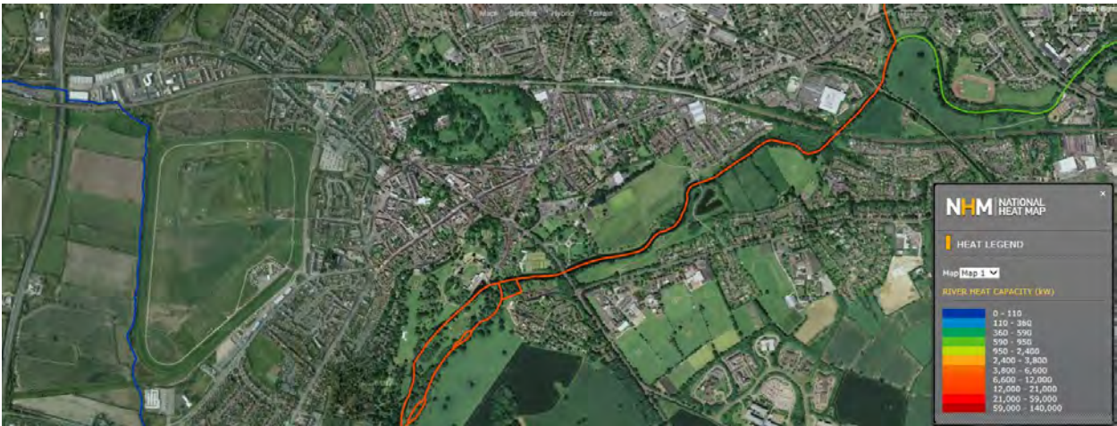
Figure 42. Extract from DECC National Heat Map showing the River Heat Capacity (in kW) near Warwick.
