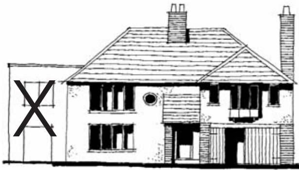
Traditional pitched roof detached dwelling with totally inappropriate flat roofed extension
