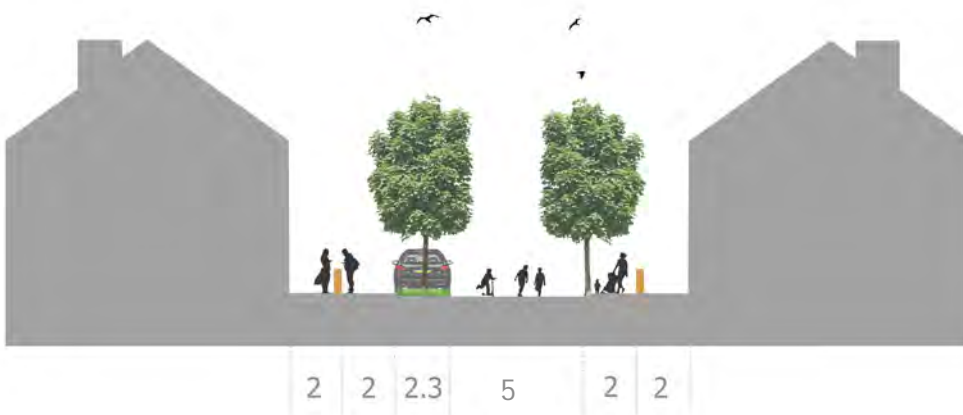
Residential Lane Cross Section (Illustrative arrangement - refer to typology parameters on page 37)
