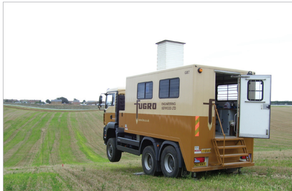
Cone penetration testing. Image courtesy of CH2M Hill.
