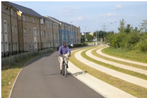
Forward visibility and curve radii accommodate commuting design, Cambridge
