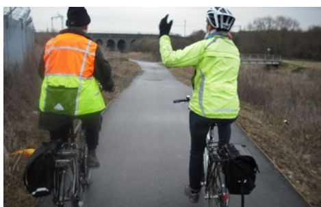
Northampton – width allows cyclists to ride two abreast with comfort (but not pass oncoming cyclists while two abreast)
