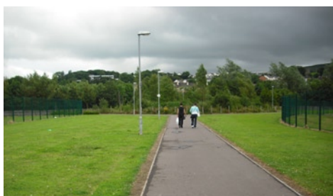
Strabane – Lighting columns installed away from path edges to maintain effective width
