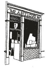
stallrisers of not less than 450mm (eighteen inches) in height. Often, a higher stallriser will provide better proportions and a 450mm height should generally be regarded as an absolute minimum.
