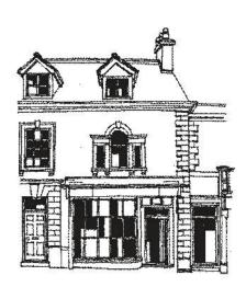
The Stallriser is the solid base of the shopfront glazing and gives protection at ground level. Traditional stallrisers can be made of wood, stone, or brick.
