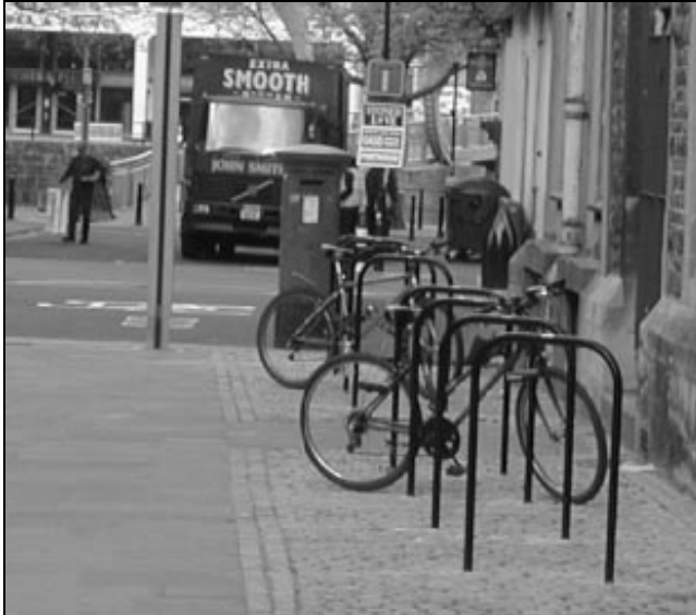
Example of Sheffield type stands (source: Sustrans Information sheet FF37)
