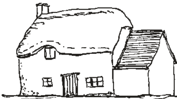
A thatched house with later addition having a clay tiled roof
