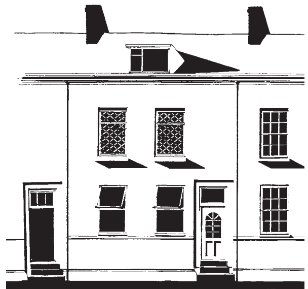
The effects of unsympathetic replacement windows and doors.
