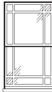
An example of an early to mid nineteenth century sash window and a french casement window with margin lights.
